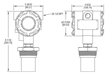
The SERIES ULT Ultrasonic Level Transmitter provides non-contact measurement of liquid levels in an explosion-proof body. It is capable of measuring up to 32.8' (10 m) with a PVDF sensor and 4 to 20 mA output.
